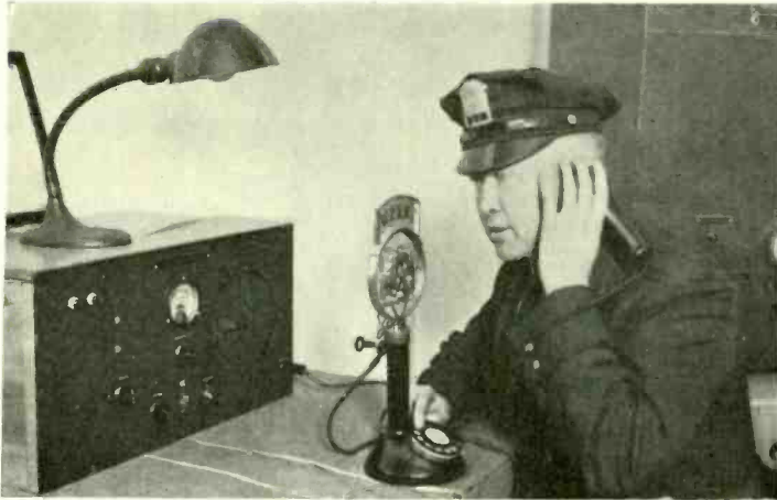
(Photo courtesy General Electric Company) Headquarters of W2XAT—dispatcher talking with "two-way" police cruiser car. Car receivers are tuned to the frequency of the headquarters transmitter frequency while each car transmitter is assigned a frequency of its own.
