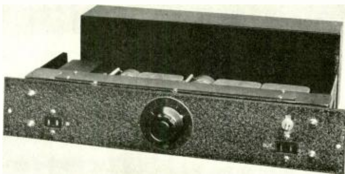
The pre-amplifier, with dust cover, for rack mounting.
