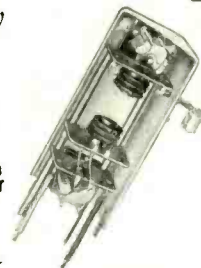
Shield cut away to show mechanism
