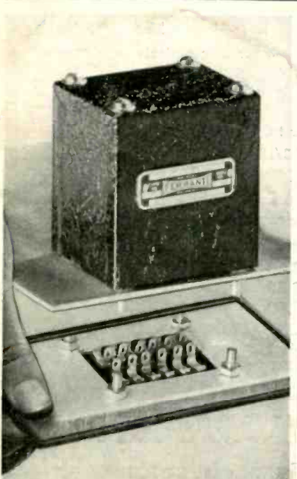
Mirror Illustrates New Sub-Panel Mounting
