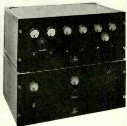
FIG. 4. (BELOW) THE SMALLER TYPE OF REDIFFUSION AMPLIFYING EQUIPMENT.
