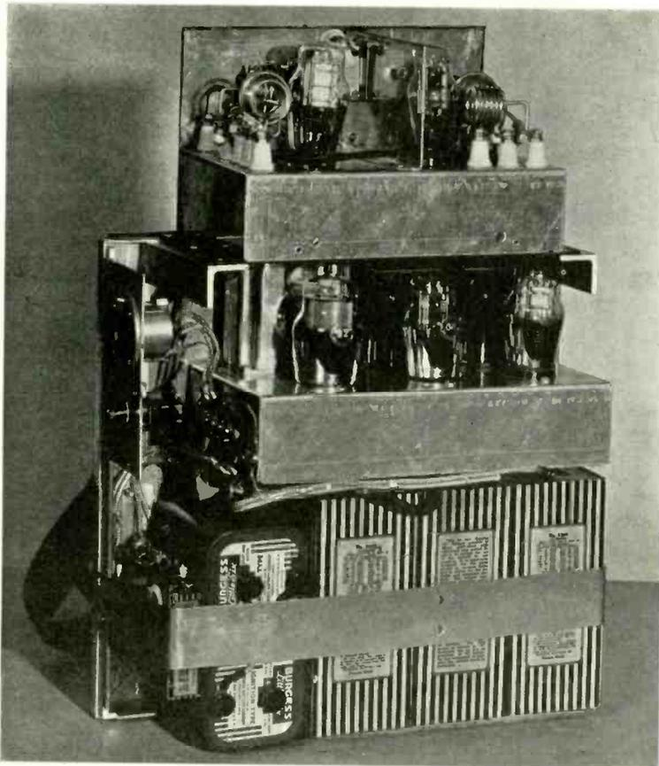
FIG. 1. SHOWING THE ASSEMBLY OF THE TRANSMITTER.
