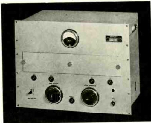
Three stage push-pull line amplifier, gain 67 db. Undistorted output plus 20 db. Response within plus or minus 1 1/2 db. 30 to 12,000 cycles. Input and output impedance is 500 ohms balanced to ground. Key provided to switch to auxiliary input. Tubes: 2 - 6A6 dual triode, and 2 - 89 triode connected. Shielded input transformer, cushioned in rubber. 100,000 ohm Remler wire wound potentiometer gain control. V.I. reference variable from minus 10 to plus 20 db.
