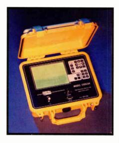
Improvements in the Model 1205CXA include sub-nanosecond pulse width, a larger liquid crystal display (LCD) and a simplified keypad. The unit also features waveform storage, wave viewing software, range-finding, intermittent fault detection, an RS-232 serial port, noise filters, automatic search capability, a rechargeable battery pack and weatherproof packaging.
