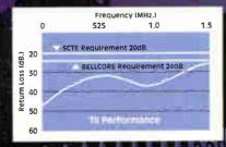
Til can handle high energy surges with very low capacitance and low arc voltage. Our coaxial protectors easily exceed both SCTE and Bellcore requirements. For more information, call 1-888-844-4720. Visit us at www.tii-industries.com.
