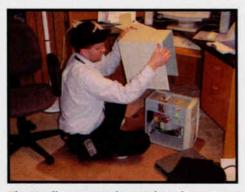
The installer removes the case from the customer's computer preparatory to installing the NIC. Before this stage, all cabling for computer peripherals (printer and so forth) should be removed and marked, and the computer should be plugged into a grounded outlet to protect against static shock.
