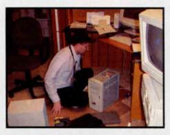
Preparing for a high-speed data install, an installer with MediaOne's St. Paul, Minn., system has moved the customer's computer onto the floor, where he has plenty of room to work, and is performing a visual qualification inspection of the unit to find an open expansion slot for the network interface card (NIC). All photos courtesy of MediaOne
