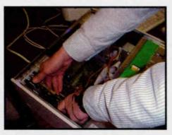
The installers inserts the NIC into an open expansion slot in the customer's computer. Note the grounding cord on the installer's left wrist, used to prevent damage to the equipment from static shock.
