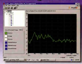
TraffiControl" measures and plots ingress spectra of bands fully occupied by return traffic
