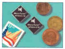
devices are single-chip, fully integrated (including low noise amplifier), dual-conversion tuners that support both analog and digital applications. Micro-Tuner chips are available with performance optimized for specific markets, including interoperable cable set-top boxes, cable modems, personal computers (PCs)/TV sets, and digital TV sets. The chips feature a 30-percent power reduction over previous series.
