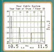
Video Output with Test Carrier Levels
