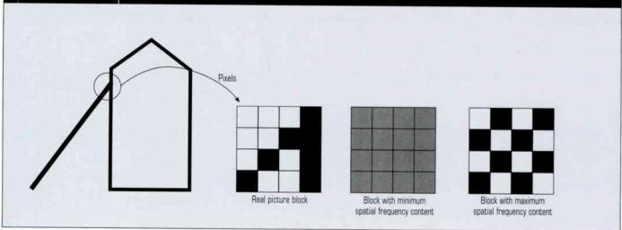
transitions per unit of time, but it is equally valid to think of frequency as the number of cycles or transitions per unit of distance. Furthermore, we don't need to restrict ourselves to thinking of frequency along just one axis: We can think of frequency along two axes, horizontal and vertical (and I sure hope I
