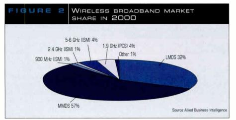
But the higher the frequency, the less likely it is for carriers to put their spectrum to use for business customers. The reason is scope of reach: LMDS and higher frequencies have a more limited range than MMDS. LMDS, for example, has a radio range of two to three miles, while MMDS has a 25- to 30-mile radius.
