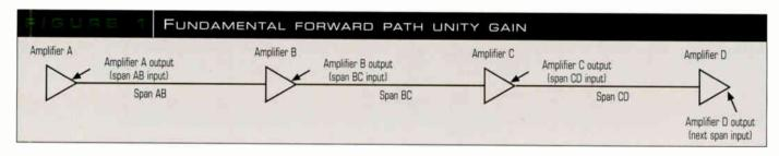
equal to the total loss of the cable and passive devices immediately upstream from that amplifier. This concept is known as unity gain, and is still a critical parameter in modern cable system design and operation.
