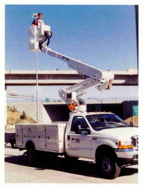
Though it looks simple, working with bucket trucks carries numerous risks, from getting "bounced" out of the bucket by an impact with another vehicle to ripping down a restaurant's drive-through awning.
