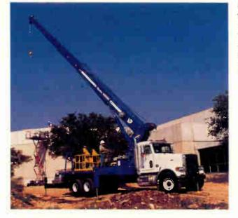
Large vehicles such as this truck-mounted crane underscore the need for welltrained drivers. Backing such a rig should be avoided if possible, but a skilled driver should be able to do so safely if necessary.
