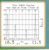
Video Output with Test Carrier Levels
