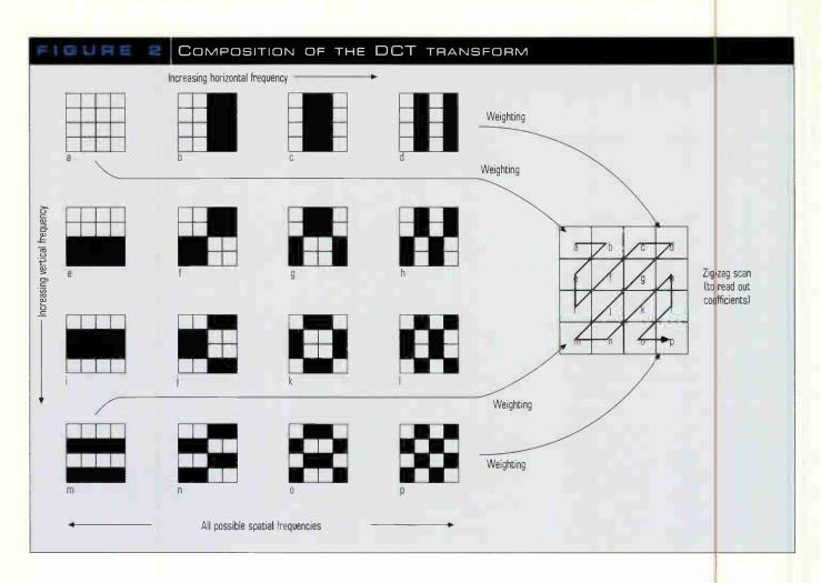
would figure out what the average value of the video is in the real picture block and assign the appropriate weighting factor to block A. This weighting goes in the DCT block shown at the right of Figure 2, at location A. This DCT block is nothing more than a way to keep track of the appropriate weightings for each of the 16 patterns in the left part of Figure 2. Just so you know, in the real world of Moving Picture Experts Group (MPEG) compression, the block is 8 x 8 and has 64 unique patterns.
