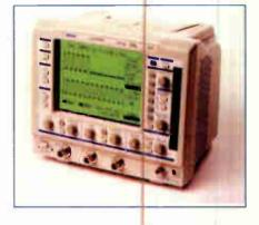
trigger, hardware five-digit frequency counter, and various automatic measurements. With built-in printer, it measures  $8.25 \times 7 \times 65$  inches and weighs about six pounds.
