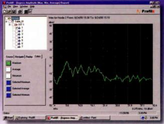
TraffiControl<sup>®</sup> measures and plots ingress spectra of bands fully occupied by return traffic
