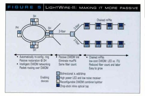
ther simplification of the network, especially when combined with the fact that digital baseband signals allow for significantly larger loss budgets. Moreover, the new components simplify redundancy switching at secondary hubs and allow for moving optical switches to primary hubs.
