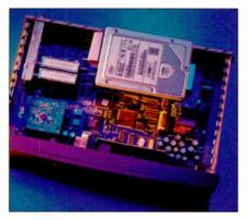
video stream and local storage in the set-top box to allow creative enhancements to content, such as highlights, interactivity and intelligent recording. The XTV Pace set-top box includes a 20 GB hard disk, allowing the device
