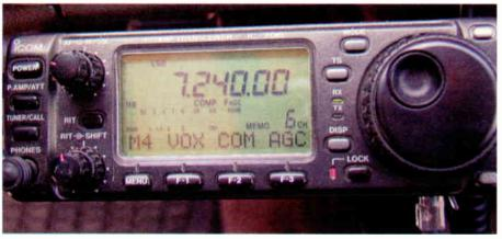
**Mobile ingress source:** This is a close-up shot of the ham transceiver in the author's Jeep. This diminutive radio (note the phone jack-type microphone connector near the lower right bottom of the radio (actually an RJ-45 connector)—can transmit 100 watts on all of the ham bands from 160 meters through 6 meters, and 10 watts on 2 meters.
