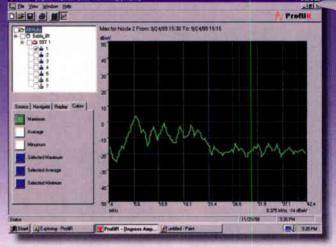
TraffiControl<sup>m</sup> measures and plots ingress spectra of bands fully occupied by return traffic
