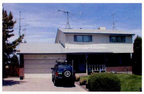
Stationary ingress source: This photo is the front of the author's house—look closely and you can count 10 amateur antennas on the roof, plus a DBS dish. The Jeep sitting in the driveway has four amateur antennas plus a CB antenna.
