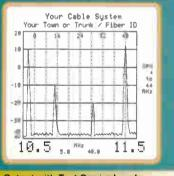
Video Output with Test Carrier Levels
