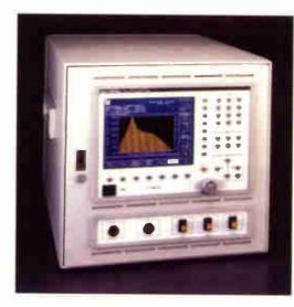
(WDM) component, amplifier and system testing. The SSB-9200 can accommodate up to 48 individual distributed feedback (DFB) laser sources for high-
