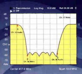
The CD-9002 will delete an entire television or LAN channel and allow a new television channel or data to be reinserted.
