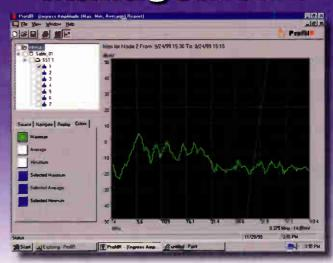
TraffiControl<sup>14</sup> measures and plots ingress spectra of bands fully occupied by return traffic
