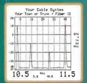
Video Output with Test Carrier Levels
