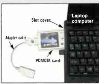
Figure 5: Inserting PCMCIA card into slot
