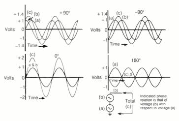
The first question then is: What is the waveform resulting when two sine waves having slightly different frequencies are added? The two television carriers are said to have *slightly* different frequencies because in general their frequency separation is small compared with their frequencies. (In contrast to the case illustrated in Figure 34 where one frequency is 10 times the other.)
