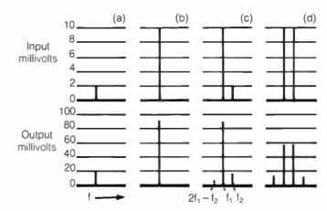
illustrate the resulting output signal components. The amplifier voltage gain, for small signal input, is 10 times. Thus, as illustrated in Figure 51(a), an input of 2 millivolts gives an output of approximately 20 millivolts.
