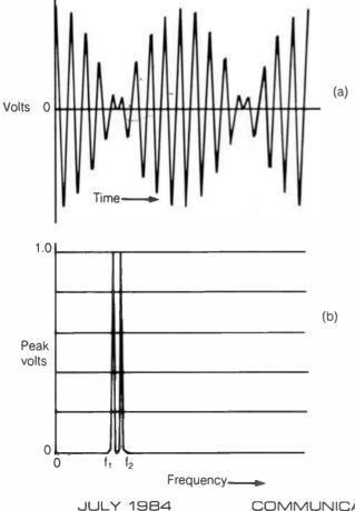
a distortionless amplifier, the output contains only the two original components, or in other words, the waveform of the output is the same as that of the input.
