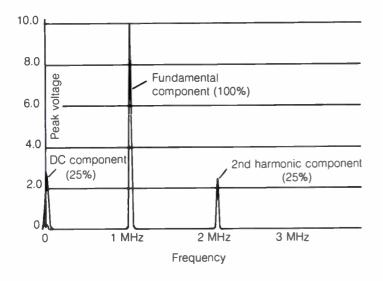
one-half cycle to its positive maximum (+2.5 volts) so the three add to produce the stretched peak of the total (+15 = 2.5 + 2.5 + 10). At 0.75 microseconds the second harmonic and the DC are at +2.5 volts so they subtract from the -10 volt peak of the fundamental to flatten the peak of the total (-5 = -10 + 2.5 + 2.5).
