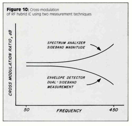
hybrids. The magnitude of the phase difference between the carrier and cross-mod sideband components can be calculated by first measuring the magnitude of the crossmodulation sidebands on a spectrum analyzer and then comparing the results to the measurement of amplitude cross-modulation by standard National Cable Television Association-sanctioned techniques.
