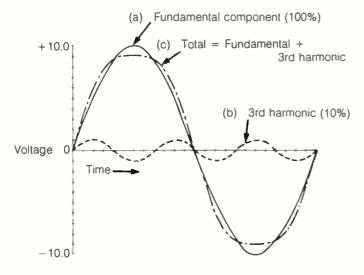
opposite in phase to the fundamental at its positive peak, with the result that the peak of the total is flattened and is again opposite in phase at its negative peak, so the peak of the total is also flattened at that time.
