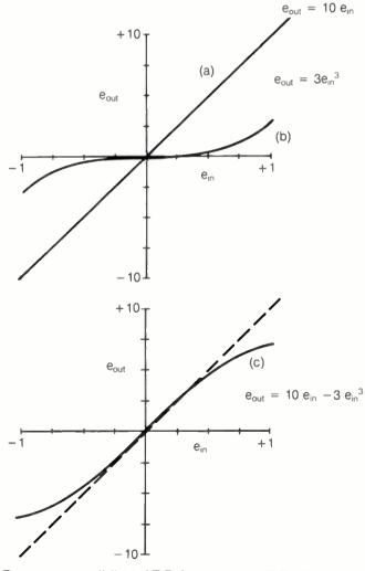
The corresponding curve is plotted in Figure 38. It is "skew symmetrical"; that is, the curve for negative magnitudes of e has the same shape as for positive magnitudes, but is upside down and has opposite direction.
