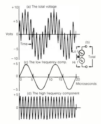
varying voltage has its most important application in the study of distortion. Earlier we discussed the distortion produced when a sinusoidal input is applied to an amplifier with second order distortion.
