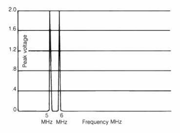
adding together equal 5- and 6-MHz sinusoidal voltages. As long as this waveform is duplicated *without any distortion* no additional components are necessary to reproduce it. A general principle relating to amplifiers can be stated:
