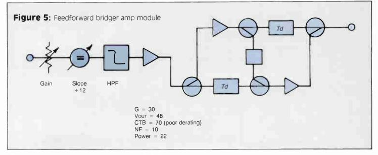
gard because there are usually many "end-offeeder" locations fed from a single bridger. Both theoretically and practically, an extra dB of output signal level at a bridger will be translated into longer reach between the bridger and the 10, 20 or more end-of-feeder locations that the bridger feeds. The longer feeder reach means lower system cost. The bridger is a natural location to apply techniques that increase the power delivered by new technologies.
