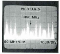
These pictures were produced wih a 4-foot diameter Prodelin dish, feeding a 63 dB gain LNA. Observe the tall Westar 5 carriers, versus the much lower amplitude Satcom 3-R signals. The view toward Satcom 3-R was somewhat limited.
