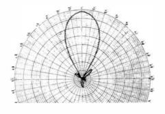
Compare these two antenna radiation patterns. The pattern on the left side has very limited directivity. The right-side pattern is much more desirable. Also note the radiation pattern nulls at 90° and 270°.
