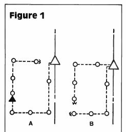
Figure 1A shows misuse of bridger port availability, and the placement of a line extender to accommodate the design. Figure 1B shows proper utilization of bridger ports and spares a line extender as well as accommodating the design.
