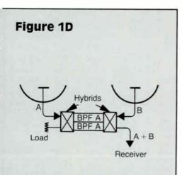
One may wish to combine (or separate) two channels. This can be done with a pair of identical bandpass filters (corresponding to one of the channels) connected between two waveguide 90 degree phase shift hybrid splitters.
