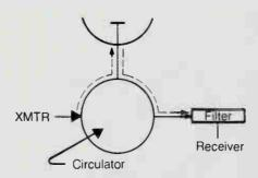
Due to antenna return loss, transmitter power may reach the receiver as shown. If the two frequencies are close, a bandstop filter is indicated, otherwise a channel bandpass filter for the receiver frequency is indicated.
