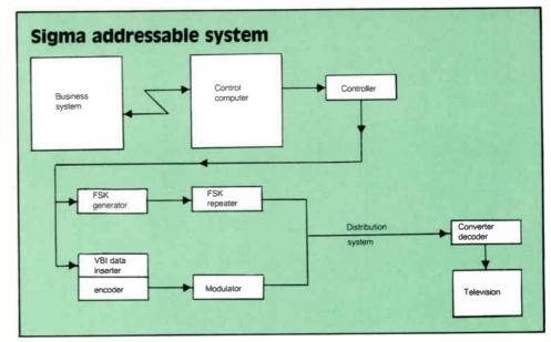
thentication information is delivered on the frequency shift keying (FSK) control channel, at 104.75 or 112.7 MHz. The control channel communicates information to both encoders and decoders. Control information must match the VBI data, creating a lock that prevents the decoder from being defeated by feeding it false information.
