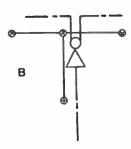
Figure 2A shows impractical designing and a waste of an amplifier. Figure 2B shows the proper placement of the amplifier in conjunction with a splitter. Note: The signal is obviously weaker in both directions in B as compared to A, however, not enough to justify the usage of an extra amplifier in most cases.
