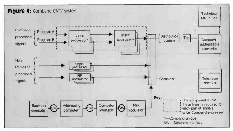
to the compressed format it provides composite 6 MHz output channels that are selectable within the frequency range of 50 to 450 MHz. Each Comband channel can be combined with all other standard NTSC channels in
