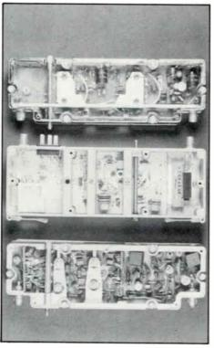
Examples of three types of amplifiers (top to bottom): a two-hybrid (quad) 400 MHz amplifier; a 300 MHz amplifier with single ended input and push-pull hybrid output; a 240 MHz amplifier with single ended input, discrete push-pull output (transistor).
