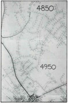
Strand maps developed from utility or telco records form the basis for system mapping.
