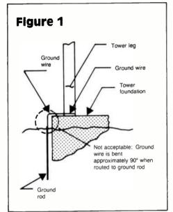
time and trouble to correct the grounding on all your towers, because it will greatly reduce the chances of damage to equipment when lightning strikes.
