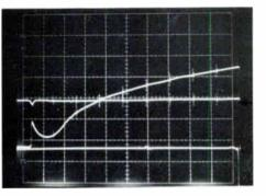
1) Return loss of a resistor-type 75 ohm terminator—30 dB at 100 MHz, 22 dB at 400 MHz. (Note: Arrow on photos indicate the reference line.)
