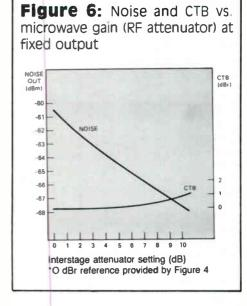
fades since the transmitter noise is attenuated along with the signal.
