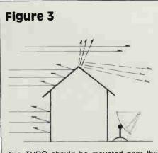
The TVRO should be mounted near the blocking screen or structure to minimize reception of microwave energy diffracted from the edge.
