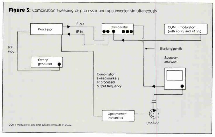
using this particular test configuration is that channel markers (visual and aural carriers) are present along with the swept response. It also shows the filter response with the adjacent channels present.
