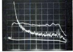
4) End of reel of coaxial cable unterminated.
