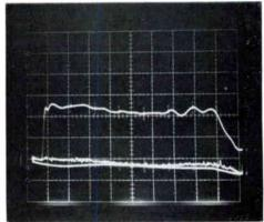
8) Variable bridge controls properly adjusted to match the average impedance of cable under test.
