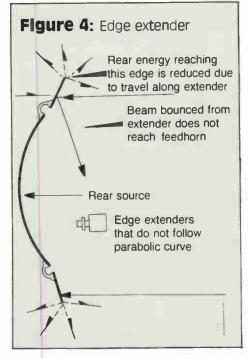
ception sensitivity of the pickup horn is reduced. Alternatively, the outer edge of the dish may be covered with microwave absorbing material (Figure 5) to dissipate the incident interference, and reduce diffraction.
