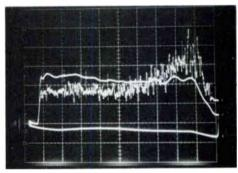
6) Bridge capacitance improperly adjusted.
