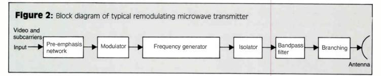
generator, an isolator and a bandpass filter. Each of these devices plays an important part in the transmission process.
