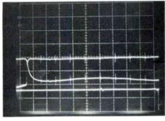
2) Using a series of high-value attenuators in conjunction with a resistor-type terminator produces satisfactory return loss (>40 dB).
