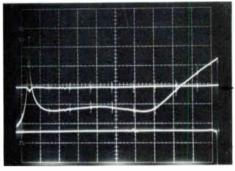
3) Return loss of the input port of a two-way drop splitter.
