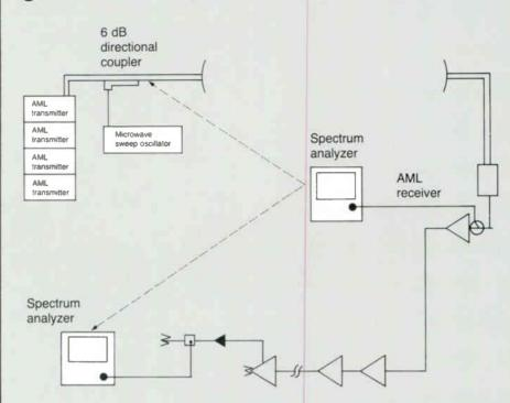
First, a mention about the Hewlett-Packard test equipment used. The microwave sweep oscillator consists of an 8620C mainframe with an 86260A RF plug-in module installed (12.4 – 21 GHz). The spectrum analyzer used was a 181T mainframe with a 8559A plug-in module for viewing the microwave frequencies and a 8558B plug-in for viewing the VHF.
