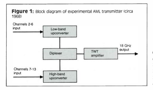
'To improve the range capability of the block upconversion type transmitter, one can trade off (composite triple beat) for power output'
