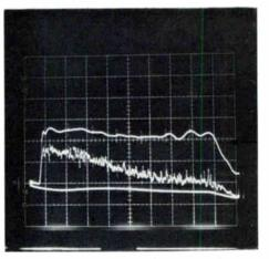
7) Correctly adjusted bridge capacitance.
