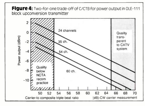
power levels summarized in Table 2, the microwave path length would be severely restricted, particularly for a large number of channels. For instance, using 10-foot antennas, the receiver input for a 54-channel application at a range of five miles is barely -47 dBm so that a standard 53 dB C/N cannot be
