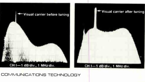
Figure 2: Upconverter response—before and after adjustment
