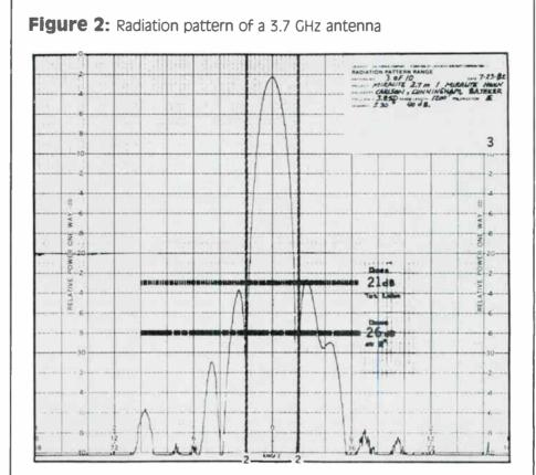
This antenna has first side lobe gain of -21 dB (relative to main beam gain). Courtesy of Miralite.
