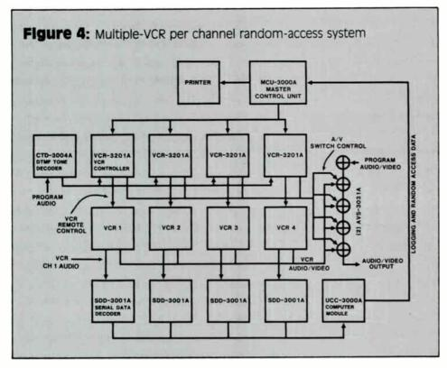
block diagram of a multiple-VCR random-access system.
