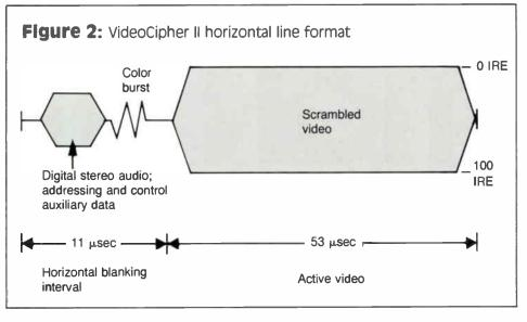
width are required. As a result, a signal scrambled with VideoCipher II shows up to a 2 dB advantage in video signal-to-noise ratio (for a given carrier-to-noise ratio) relative to an unscrambled signal.
