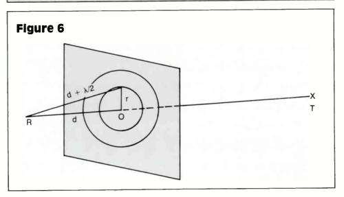
screen to the receiver is  $d_2$ , then the general expression for the radius of the n<sup>th</sup> Fresnel zone is  $(n\lambda[(d_1 \times d_2)/(d_1 + d_2)])^{1/2}$ . The radius of the first Fresnel zone is  $r = (\lambda d_1 d_2/D)^{1/2}$ , where  $D = d_1 + d_2$  and all the quantities are expressed in the same units.
