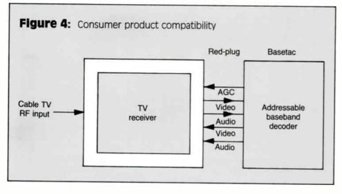
VCR can be designed to interface with a lowcost external or internal addressable baseband descrambler. This approach returns the channel tuning function and other features to the consumer's TV product where they are the most effective.
