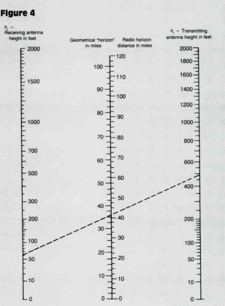
Nomogram giving radio-horizon distance in miles on a smooth spherical Earth when h, and h, are known. Example: Height of receiving antenna 60 feet; height of transmitting antenna 500 feet; maximum radio-path length = 41.5 miles (K = 1.33).
