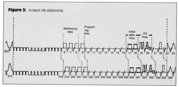
mission. This being the case, addressing data either is transmitted along with program tagging and decoding information as aural carrier amplitude modulation or is transmitted in an out-of-band data channel. Each method requires a separate data receiver in the home terminal and can either cause undesired audio by-products or use up valuable CATV RF spectrum.
