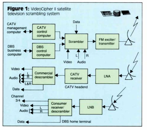
given program transmission, it reverses the steps performed at the scrambler to produce video, three audio outputs (left, right and mono), and the auxiliary data signal.
