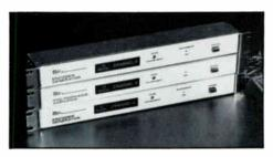
Model LS-(channel) lower adjacent security module, an optional accessory, is used when the lower adjacent channel is unoccupied by programming. It generates an RF signal at the lower adjacent sound frequency making it impossible for subscribers to fine-tune in part of the premium programming.
