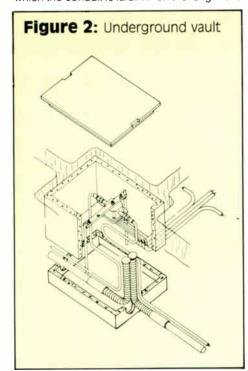
conduit section exceeds the allowable limits, a manhole should be provided in the curve or the manholes adjusted to shorten the section.
