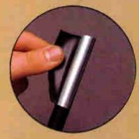
Jacket bonded to sheath for additional handling ease and increased corrosion protection. Peels away easily, leaving no adhesive residue. Continuous conductor-through-jacket bonding greatly increases sidewall and pull strength.
