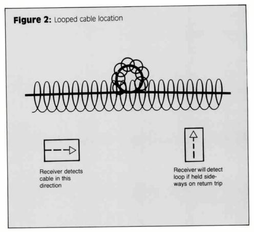
can be the result of a less than honest contractor who, being paid by the number of feet of cable placed in the ground, will loop the cable in a circle to make more money. It also
