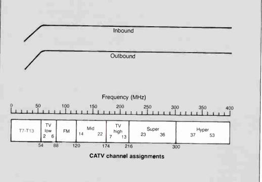
The available bandwidth for dual-cable topologies is shown. Because the cable is looped back at the headend, the full frequency spectrum is available for return (inbound) signals.
