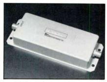
wanted signals from travelling on the return line in dual cable systems while allowing the rest of the band to pass. Insertion loss is 2 dB maximum (10-300 MHz), rejection is 40 dB minimum (DC-8 MHz) and impedance is 75 ohms. It comes in a case 1 inch x 2 inches x 6 inches with type F connectors. The cover has flanges with holes for indoor mounting.
