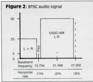
The recovery pilot, phase locked to the video-sync information, is carried at 15.734 kHz. This multiplexed signal requires a bandwidth of 46.5 kHz, and causes a carrier deviation of 50 kHz.
