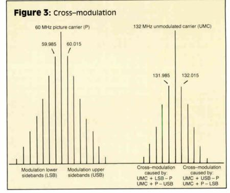
Remember, we must add 6 dB to the IM level, because triple beat is 6 dB stronger than two tone third order, which will give us a total of 18.5 dBmV IM, or referenced to the 50 dBmV input signal, 32.5 dB down.
