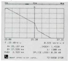
In the automatic splice loss mode, the amount of loss at the splice point is accurately measured to within 0.01dB and is instantly displayed on the CRT. Only a single marker is required to establish the splicing location on the CRT. This location is maintained going from fiber to fiber. No reprogramming required. The real-time display acts as a "live monitor" so that fiber core alignment can be optimized for minimum loss.
