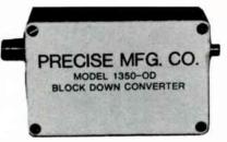
The PRECISE Model 1350-OD, Outdoor Downconverter is designed to be used with an LNA to provide a 270 - 770 MHz block down conversion of the 3.7 - 4.2 GHz satellite TVRO signal.
