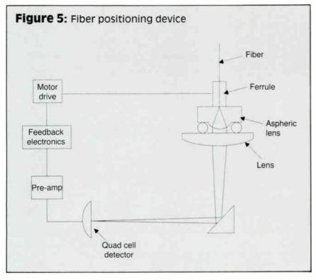
device that was transportable, usable in a field environment, and with automatic positioning capabilities of  $\pm$  0.0001 mm over a 1.0 mm range with little or no backlash or friction. Figure 5 shows some of the design elements that will be described.
