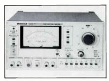
of less than 1 percent THD, this instrument will complete the measurement, eliminating almost all manual tuning. It also features S/N measurement and AC signal level measurement capabilities.
