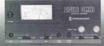
Operating functions including MGC, AGC, AFC, level sets, normal/invert video, clamp/unclamp video, status subcarrier frequency selection, video of the status are conveniently located on the montpart of the result C/N ratio, signal strength or contention
