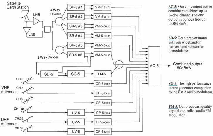
line of saw-filter broadcast equipment.
