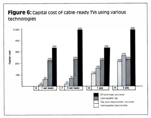
As can be seen by the comparison graphs (Figures 5 and 6), the effect of various applications can show dramatic variation in capital cost depending on technology employed. In comparison of Columns A and B:
