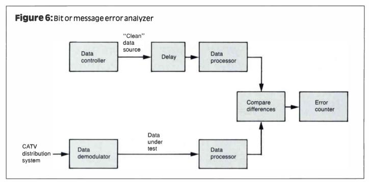
some bit errors. A particular system bit error counter may show six bit errors in a one-minute time period or 0.1 errors per second. If the data transmission rate is 10,000 bits per second there is one error for every 100,000 bits, and the BER is expressed as  $1 \times 10^{-5}$ .
