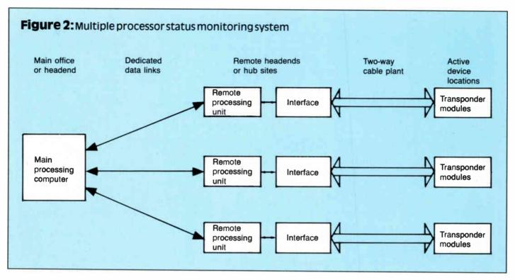
ing and controlling a number of functions. Table 1 highlights many of the monitoring and controlling features available. These capabilities can provide a cable operator with tremendous flexibility, and a well-planned status monitoring system actually will help to reduce plant maintenance costs. A cable operator can monitor the operational status of the entire cable system, immediately identify and locate problems, and remotely
