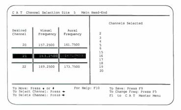
will be offered a choice of four built-in frequency plans: NTSC, HRC, NTSC+12.5, and NTSC-12.5; after which the channel numbers and the video and audio carrier frequencies will be displayed.
