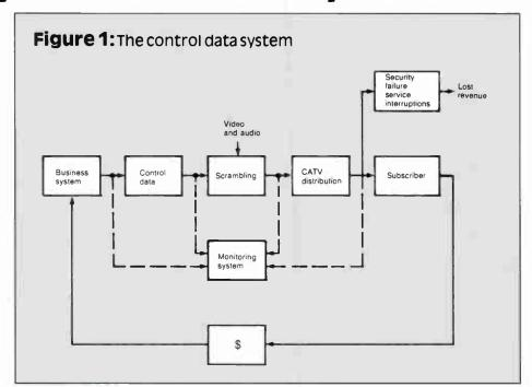
upon command is a fundamental requirement of an addressable system. Thus, control over the descrambling decoder is the control data system's primary purpose. Interface to a business system for billing purposes and control of pay features and other services are
