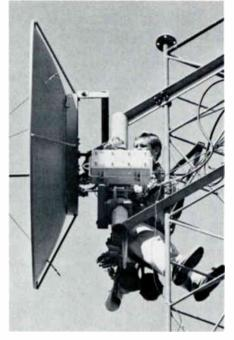
In addition to extra power, the 5-watt system utilizes GaAs FET amplification, highly stable microwave oscillator and redundancy of key components to insure reliable operation and reduce maintenance. A Status Monitor Panel, included with the 5-watt transmitter, allows remote monitoring of all system functions by
