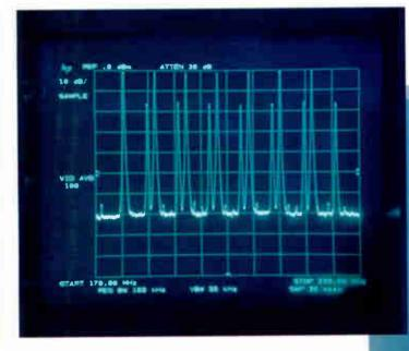
Spurious Outputs: - 60 dBc Composite triple beat: - 60 dBc Cross Modulation: - 60 dBc Output Level: + 50 dBmV Carrier/Noise > 60 dB
