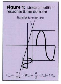
The DC variable normally is not considered in frequency amplification devices and should be considered as zero. This would leave the simplified expression y = mx or  $E_{out} = AE_{in}$ . In Figure 1, the output level is predicted by the slope of the transfer function line multiplied by the input level. This indicates input signal amplification with no distortion.
