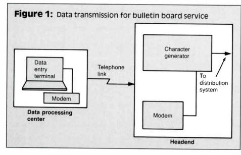
modem for transmission back to the field for analysis. The information can be transmitted by telephone, or an RF modem can interface directly with the existing cable. The signals at the output of the modem are combined with the headend signals. The receiving system extrapolates and converts the information and transfers it to a printer for immediate analysis or to a computer for storage.
