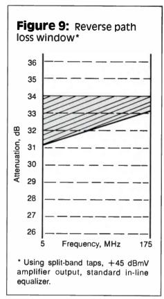
the system. The designer was able to reduce the cost of the system by improving the tap-toamplifier ratio from 10 taps per amp using standard CATV technology to 18 taps per amplifier using the split-band tap unit. The cost reduction was due to the reduction in the number of amplifiers in the system.
