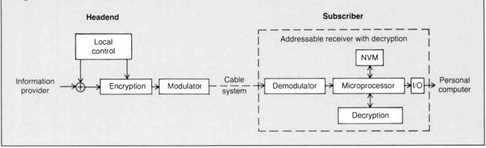
cess to the data. Unfortunately, the receiver needs to know the key that was used in the transmitter so it can decrypt the data. So, keys must be sent down the cable to the appropriate receivers. The keys must be encrypted using keys known by both the transmitter and receiver. They should be changed as often as practical.
