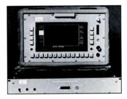
then set up specific guard bands around the carriers to protect them from any sweep interference. The receiver reads both the sweep and carrier levels, integrating them to create a high-resolution (better than 0.25 dB) sweep response.
