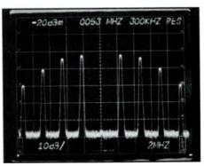
First carrier Bessel null indicates proper deviation.
