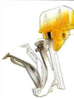
Our unique eight-point suspension and hinged drop chute with removable gate isolate vibration from the machine and cable. Service loops can be restrung without cutting or splicing. And only Case offers a front trencher, rear plow combination.
