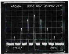
As deviation is turned up, sidebands appear, spaced at integral multiples of the modulating frequency (2.33 MHz).
