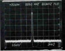
Waveform of an unmodulated carrier.
