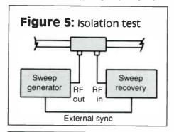
dent, it is best to sweep the device with a sweep generator or a sweep recovery system. The instruments used to align and balance the system can be used efficiently to perform tap isolation tests.
