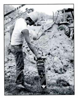
33 kHz transmitted signals. This combination is said to give precise location with or without using the transmitter. The product is equipped to give depth measurement of 10 feet.
