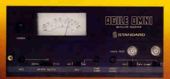
Operating functions including MGC, AGC, AFC, level sets, normal/invert video, clamp/unclamp video, skew, subcarrier frequency selection, video and IF test point are conveniently located on the front panel. Meta-multi-C/N ratio, signal strength or center-tune.
