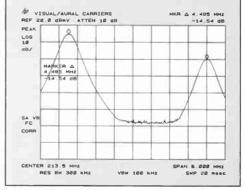
now can be used. The only limit to using FFT techniques lies in the sweep time necessary to take a measurement. The sweep-time range of the spectrum analyzer is related to the frequency range of the modulation that the FFT can measure.
