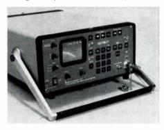
Laser Precision's high performance TD-9920 has shown outstanding reliability in the field for the past five years with the telcos, military, cable installers, and power utilities. This compact, 25 lbs., multimode optical time domain reflectometer offers more features and better accuracy than any other small portable. Designed to go anywhere, the TD-9920 operates on rechargeable battery or 110/220 VAC.
