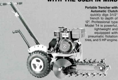
Designed for sprinkler installation it is also suited for underground cables and gas lines. It is built with the professional in mind, but because of its simplicity of controls, ease of operation and compact size it is well suited to the homeowner as well. The Ground Hog Trencher features oversize pneumatic tires, heavy duty steel fabrication, ball and timken bearings through-out, easily replaced hardfaced blades and a screw conveyor to deposit cuttings at the side of the trench.
