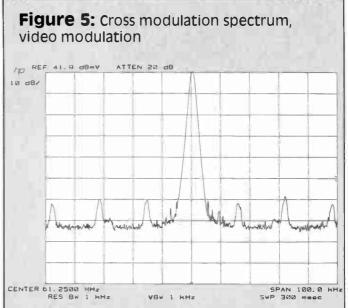
riers that produced it. The composite beat has a carrier coherent with the desired video carrier and modulation of the beats produce 15.75 kHz line-frequency sidebands. The result appears the same as cross modulation except that in this case the sidebands are present without the carrier for the channel under test, and by definition these cannot be due to cross modulation. These sidebands are evident in Figure 6.
