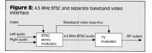
a stereo-capable television), decode the BTSC stereo into left and right audio, and output the video channel to the television. Some adaptors include a stereo amplifier and speaker connections, while others interface with the auxiliary input of an external amplifier. As well, some include a variable RF tuner for off-air BTSC reception.
