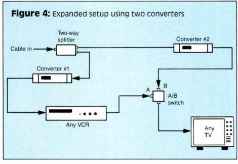
items to be considered at this time are personal viewing/recording preferences; the specific hardware to be configured; ease of operation; remote control capabilities; performance tradeoffs; and any inherent costs associated with "making it all work together." In addition, whether the system's premium services are trapped or scrambled also has an immediate impact on how the hardware is to be configured.
