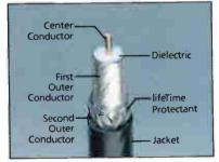
A cutaway of lifeTime\*\* cable.
