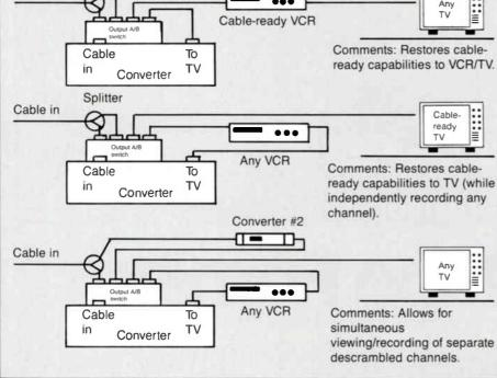
remote control using the A/B switch button. This then returns full use of a television's cable-ready capabilities by making the converter transparent to the system when scrambled channels are not involved. Several potential uses are illustrated in Figure 6.
