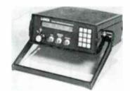
Digital (DTDR) Test Mode: Standard on all models-Pressing key "4" on the Keypad will cause the Digital Test Mode to run a one time test of the cable and display the cable condition as: "OPEN", "SHORT" or "OK TO" in feet, metors or nanoseconds.
