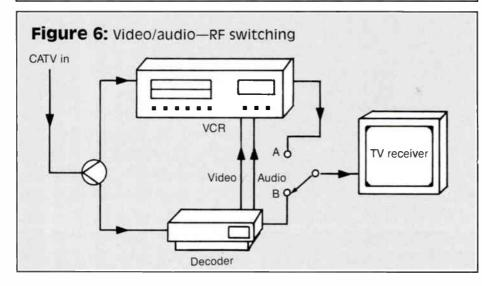
ranged in such a way that while any program (basic or premium) is being recorded, any basic program can be viewed. The VCR, however, still is only capable of receiving the CATV decoder's output channel and is incapable of programmable channel change. Operation of the system now begins to become complicated due to the addition of the manually operated A/B switch.
