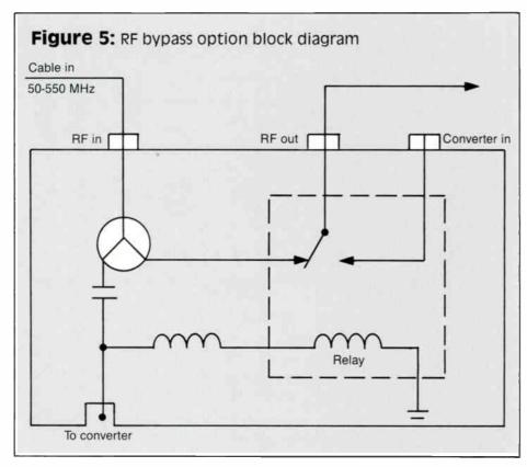
Playback of a prerecorded VCR tape is accomplished by tuning the converter to the output channel of the VCR and tuning the television to the output channel of the converter. For all other recording/viewing scenarios, the appropriate channel is tuned on either the VCR or the converter with the television tuned to the output channel of the converter. Unattended program recording also is possible on all the clear channels that can be selected with the VCR tuner.
