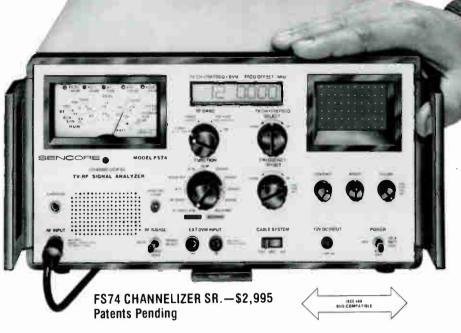
At last, a TV-RF Signal Analyzer designed the way you've always wanted it . . . Meet the world's first 100% automatic FCC accurate field strength analyzer. It's exclusively designed and guaranteed to help you analyze and pinpoint any RF video trouble, in any video distribution system in one-half the time. At long last you can accurately check your signal "quantity" and "quality"—all automatically. Here's why . . .
