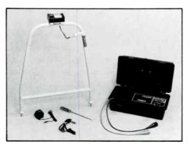
**MODEL 2003 Ground Fault Locator**
