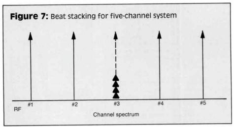
the transmission bandwidth to the highest octave region will cause all the second orders to fall above or below the desired transmission spectrum (Figure 6). Without the second-order limitation, third orders will be the limiting distortion mechanism.
