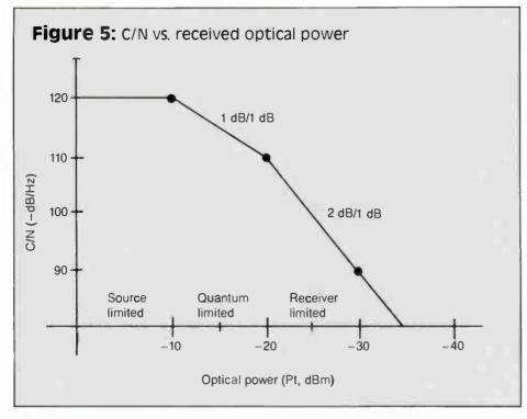
Here, C/N is directly proportional to the square of the average optical power. Thus, for each 1 dB change in optical power received, the C/N ratio will change by 2 dB. For larger optical signals incident on the photodiode, the quantum noise associated with the signal detection process dominates (assuming I<sub>d</sub> negligible), so that
