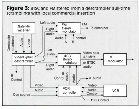
sion stations. Total BTSC signal bandwidth with all carriers, including SAP, exceeds 100 kHz and peak deviation is 73 kHz. (These specifications will take on greater significance when we discuss interfacing the BTSC encoder with TV modulators.) It should be noted that as SAP and PC are added to the BTSC stereo signal, the potential for signal degradation increases. Therefore, these signals should not be added to your system unless needed.
