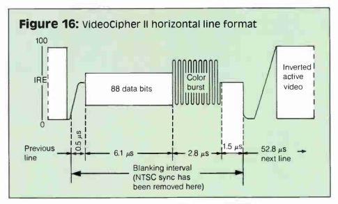
one line than on the preceding line. This either advances or delays the start of each line, producing a slewing of the individual lines. No data is omitted, it merely is sent in advance or saved for later. It is this sequence of advance/delays that is encrypted and as before, the encryption/decryption algorithms can handle this rate.
