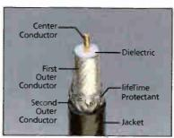
A cutaway of lifeTime\*\* cable
