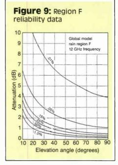
With satellite at 85° W.L., solution of this equation yields an elevation angle of 49°. From Figure 6, rain attenuation is 5.1 dB for 99.95 percent availability.
