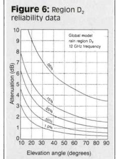
Equation 6 is the expression that a designer of a receiving earth station has to work with. He must know the satellite EIRP for the site. Satcom K1 EIRP footprint is given in Figure 10. He can then determine what size antenna to use for a desired S/N and reliability.
