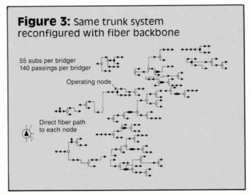
There is another benefit for systems dealing with data transmission. With a fiber path running to every part of the system and since fiber is capable of operating bidirectionally, there is a very reliable path back to the headends to carry a large amount of data. How real is this plan? Consider a little history as well as present-day developments.
