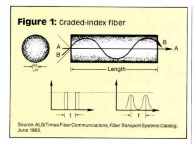
the latest arriving light from the first pulse and the earliest arriving light from the second pulse, due to the varying path lengths (see Figure 1). This phenomenon produces a bandwidth/distance limitation in multimode fiber similar to roll-off in CATV cable. In FM-based systems, this limits the total channel capacity of the fiber and is the major reason that early CATV fiber systems were limited to four channels per fiber.
