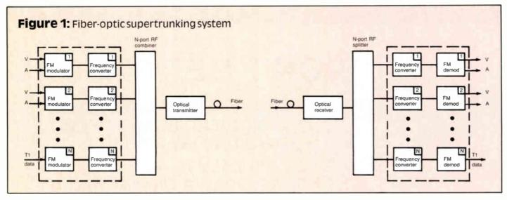
A fiber-optic supertrunk delivery system offers wide bandwidth, low losses, very small size and weight (and therefore many fibers can be packed into a small space), security of communications and rapidly dropping cost. Because of these factors the system designer can select the frequency plan, the modulation method and the number of fiber links offering the best and the most economical way of packing the number of required channels into a fiber-based supertrunking system.
