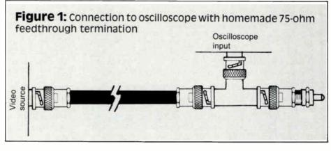
thing to remember about using a general purpose oscilloscope for video measurements: The impedance of the oscilloscope is not the same as the video source being measured! An oscilloscope has a very high input impedance typically around 1 million ohms. Most video sources have a 75-ohm impedance. Because of this, you must use a 75-ohm feedthrough termination at the input of the oscilloscope when measuring video signals.
