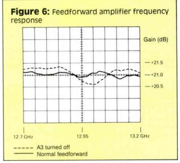
off from its normal output level. The difference in level between the feedforward input and the line extender output represents the permissible loss, which might take the form of a long waveguide run if the feedforward amplifier is to be tower-mounted to achieve the greatest possible path length. With this allowance, the line extender might still be at the base of the tower, where maintenance should be much easier.
