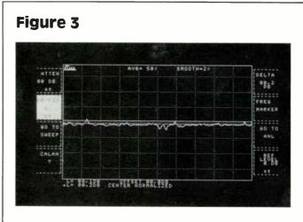
the rescue. The latest version of a system sweep uses a programmable generator that ''selectively'' places the sweep reference points around the carriers. As it turns out, this works as well for an FM trunk as it does for a standard AM trunk, with a bit of careful setup.
