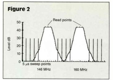
thing very irritating about limiting your maintenance resolution to every 14 MHz or so across the band. And it still does not solve the problem of the frequency response beyond the carrier locations. Eliminating a gap of 14 MHz can show some very neat frequency response variations that simply will not be seen when reading just the carrier levels.
