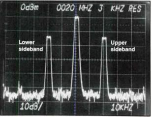
A 20 MHz carrier amplitude modulated by a 20 kHz signal. The percent of modulation in this example is about 40 percent.
