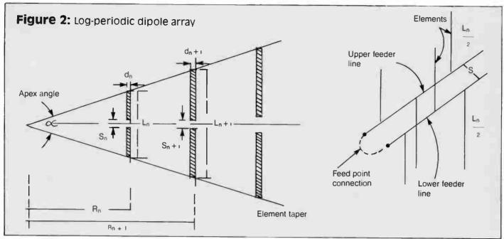
spaced farther from one another and located toward the rear of the antenna structure.
