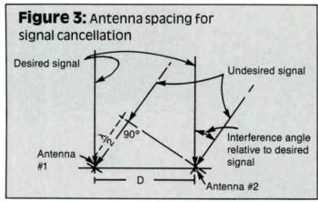
On-axis signals induce equal voltages that appear at the input ports of the signal combiner in phase and add within the combiner. This method is effective at eliminating horizontally originating reflections when the antennas are spaced in a horizontal plane. The same effect is successful at eliminating vertically traveling signals when the antennas are separated in a vertical plane. For a known angle the required spacing distance (d) is determined from the equation:
