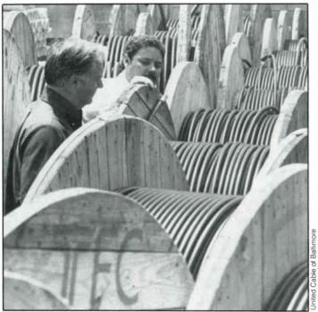
When cable reels are moved into a warehouse, they should be positioned so they are not lined up with two reel flanges meeting.
