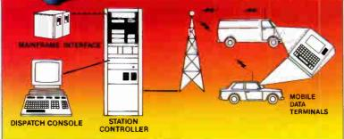
The C•ARDS System - the dispatch console includes a microcomputer which houses specially-designed software, terminals, keyboards and printers. The station controller contains equipment which interfaces the microcomputer to your billing system and existing radio base station. Mobile data terminals in each vehicle enable operators to communicate with the dispatcher, send information and access data stored in the microcomputer or a host computer.
