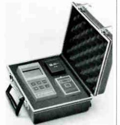
If used for LAN applications, the loss test set includes: the AM-3500, built-in Silicon detector, rechargeable battery, AC adapter, earphone, choice of adapter for any multimode connector, and a bare fiber adapter, hardshell carrying case and soft packs, plus a AP-3200 LED 820nM hand held light source. The price for this complete loss test set is only \$1,590.
