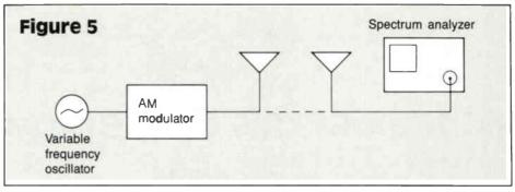
"The total harmonic distortion...can be determined by noting the amplitude difference between the modulation signal and its harmonic products."
