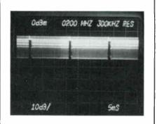
• Tune to the channel being measured using the "center frequency" control and adjust "input attenuation" and "reference level" controls to produce a display similar to Figure 1.
