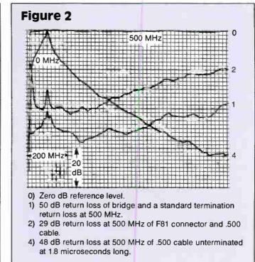
with TSSRL. The high sweep speed and narrow IF bandwidth will reduce the effect of other signals that are on the system and enhance the desired signals.
