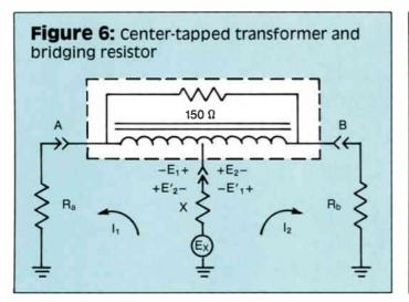
design for many people is the means by which isolation exists between ports A and B. The nature of this isolation is easily explained. Referring to Figure 7 we have the same design as in Figure 6, but with the generator ( $E_A$ ) placed in series with  $R_A$  (one of the two 75 ohm load resistors) rather than  $R_x$ .
