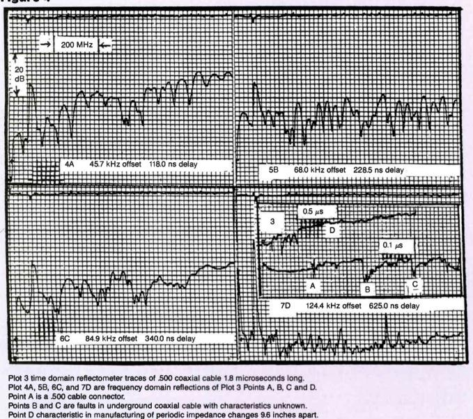
is made after a tracking offset change has been made. The midsweep output frequency difference is the offset. The frequency offset of the tracking generator will determine the spectrum analyzer time delay.
