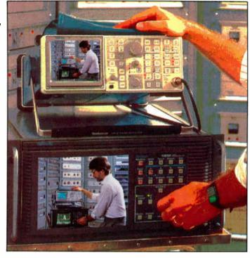
measurement set was developed by Tektronix Inc. Complete analysis of video can be made using its integrated digital waveform monitor, digital vectorscope, noise measurement set, group delay measurement set, automated monitoring system and automated measurement set. Figure 1 shows a (reduced) hard copy of detailed analysis of a demodulated (a Tektronix 1450-1 precision demodulator with TDC-1 tunable downconverter was used for all tests) off-air signal on Ch. 18
