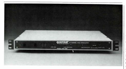
Fully agile, Qintar's AVM-7060 offers output channel selection of VHF 2-13, midband A-I, superband J-W, A-1 through A-6, and hyperband AA-WW. In addition, the AVM-7060 offers a front panel FCC offset switch for FCC required 12.5 kHz or 25 kHz and a rear panel switch for standard, HRC, and IRC offsets.
