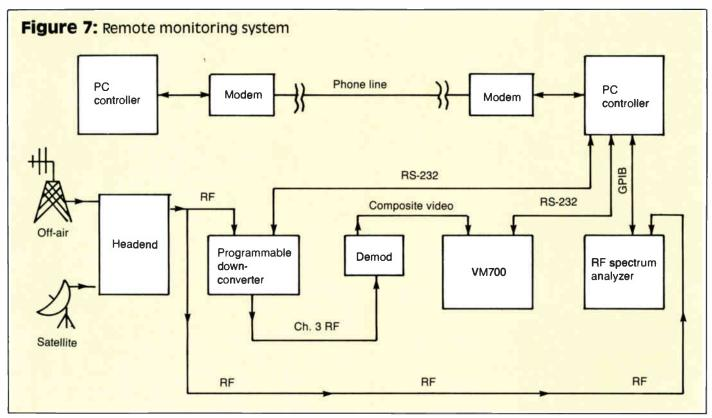
component is suspected to save time and possibly another tower climb—wire is cheap compared to an accident), again the dBmV level from the RF spectrum analyzer should be recorded, and the S/N level noted with the VM700. If unsatisfactory noise figures still exist, the antenna needs to be: repeaked for best location within its polar pattern, raised (noting free-space benefits), relocated to prevent the desired signal's energy from being affected by nearby antennas or replaced.
