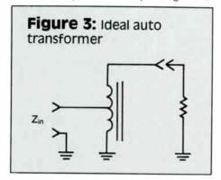
off not found in other applications of this circuit. The property of the core material, most responsible for signal transmission, is called *permeability*. Unfortunately, at 300 MHz, this permeability decreases to almost nothing.
