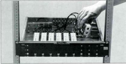
If you've ever had to add or change a channel on your headend in the field, you know how difficult and time consuming it can be. On the other hand, our new *modular* Geomax-10 processing system makes the job a snap. You just plug in a new module. Each of the 10 modulators or processors is a mere 25 cubic inches in size and weighs less than 1 lb. for easy shipment and handling. Our completely modular approach, coupled with a second standby power supply and ultra-lightweight construction make the
