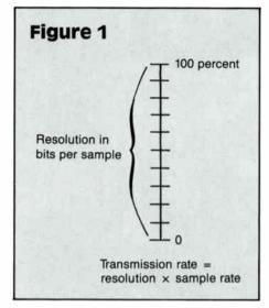
observed when the signal is converted back to the analog format. For example, a fixed video scene that gradually changes in shade will be observed to have abrupt shade change boundaries instead of a smooth transition. Correspondingly, if the digital sampling rate is not adequate, then changes in picture content will not be accurately reproduced; i.e., motions will appear to be jumpy.
