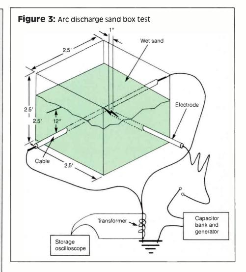
Siecor armored Mini-Bundle cable (copolymer-coated ECCS steel armor): No significant damage occured to the inner sheath and no core damage occurred on this design tested to 115 kA. Only the outer jacket and armor was penetrated at current levels as high as 150 kA. At higher levels, to 229 kA, only minor damage occurred to the inner jacket and again no core damage occurred.
