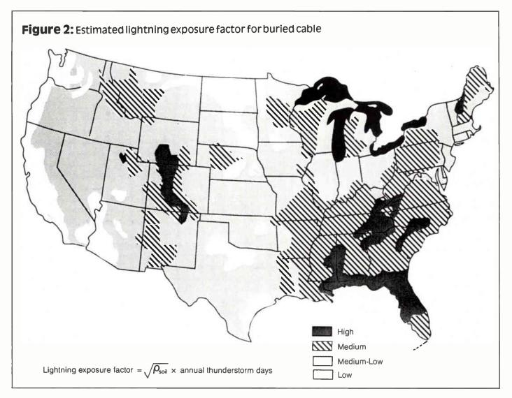
stand very high levels of surge current. The cable's ability to quickly dissipate this current following a lightning strike helps to minimize the damage caused by further arcing, burning or charring.
