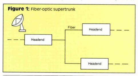
cable. Two alternatives are available for the deployment of FM supertrunking. The simplest is to divide the cascade in half at the midspan amp (36th amp in the previous example). A supertrunk link is virtually transparent so that for all practical purposes the performance at the input of the 36th amp is the same as that of the headend. At the end of the line C/N has improved to 46 dB, with CTB improved to nearly -59 dB.
