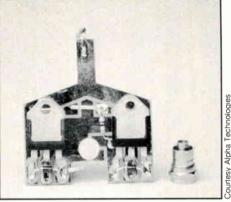
The AmpClamp shunts coax to sheath within a few nanoseconds.
