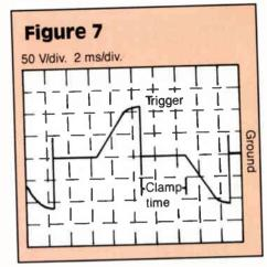
could get rid of. The voltage across the SCRs when conducting is only 0.3 volts. It does not even show as such in Figure 7 where you can see an overvoltage of about 220 V instantaneous taken to within 0.35 volts of sheath ground in a matter of nanoseconds.
