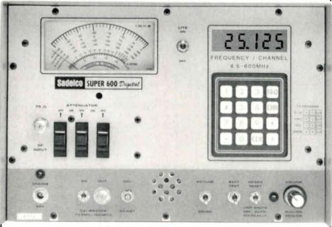
Model Super 600 Digital Signal Level Meter
