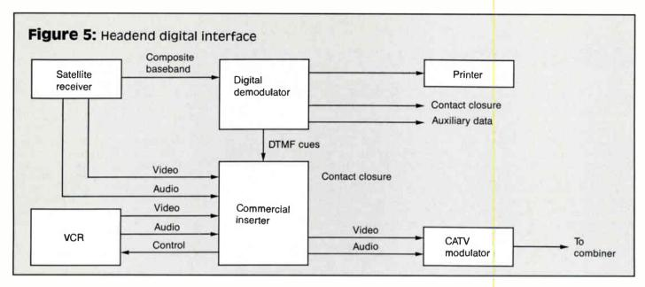
cuitry is a part of the ad inserter and two momentary DTMF cues are used rather than a closed relay.
