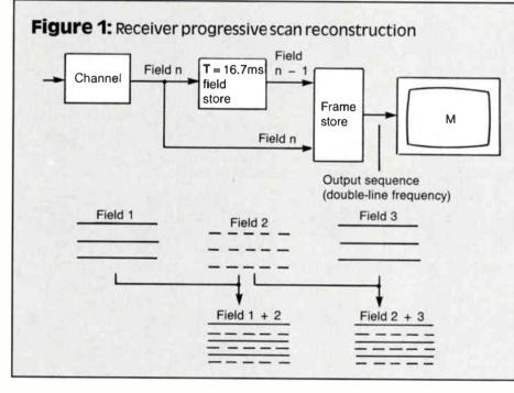
originally progressively scanned and sent as previously described. However, this technique would suffer artifacts due to motion if applied to a signal that was generated by an interlace scan. In that case added logic can be used to interpolate between successive lines in a field to generate the other interlaced field.
