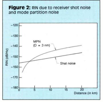
mechanism that affects all modes equally will not affect the MPN, since the cancellation will not be affected. Conversely, any mechanism that transmits the modes unequally will tend to destroy the cancellation, causing an increase in laser noise.
