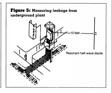
on connectors and the new A/B switch rules will test our skills. If a pre-wire has poorly shielded cable there is a potential for leakage. Where there are store-bought or push-on connectors installed by do-it-yourselfers, there is potential for leakage. Where there are A/B switches, there are more fittings and more potential for leakage.
