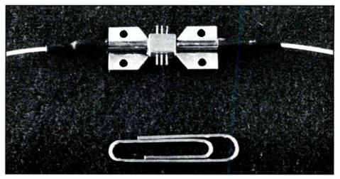
The diode laser amplifier is the only optical amplifier commercially available.
