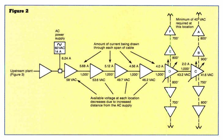
for any eventual additions to the system and the AC power supply will not have to be relocated. Also, it is not wise to allow more than about 6 A of current to flow through any amplifier. Of course, this applies mainly to the amplifiers closest to the AC supply.
