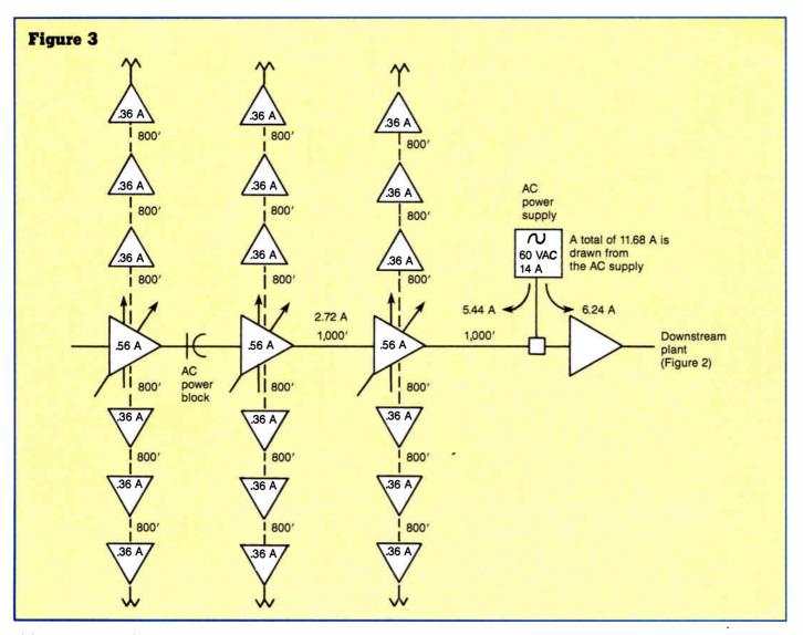
plying 1.5  $\Omega$  by 0.72 A we calculate a drop of 1.1 V (rounded off). The required output voltage at the bridger/trunk is 41.6 VAC. Keep in mind, we are working upstream toward the AC power supply location so that the voltage levels at each amplifier will increase.
