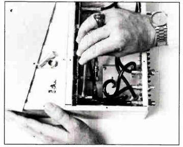
Step 9: Wrench tighten the connections then repeat Steps 4 through 9 on the other internal chassis connectors.
