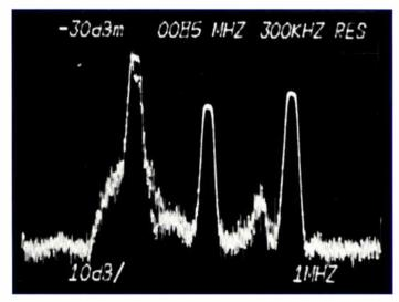
**Photo 1:** While observing the processor's RF output on the spectrum analyzer, tune the sweep generator's CW signal to the center of the channel being measured and adjust the level of the sweep signal 2 or 3 dB below the sound carrier amplitude. This will prevent the sweep generator from interfering with the processor's AGC.
