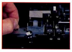
**Step 7:** The Type-35 automatic fusion splicer only requires selecting a splicing program from a menu on the self-contained monitor, placing the prepared fiber into the clamps and pressing the start button to initiate the fusion splicing procedure. The microprocessor controls the entire process.
