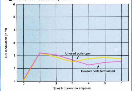
Figure 8: Test results of Tap A and Splitter A
