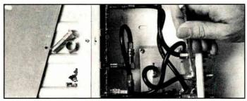
**Step 10:** To replace an external chassis connector disconnect the RG-59 jumper from the connector. Check the cable's center conductor diameter and length.
