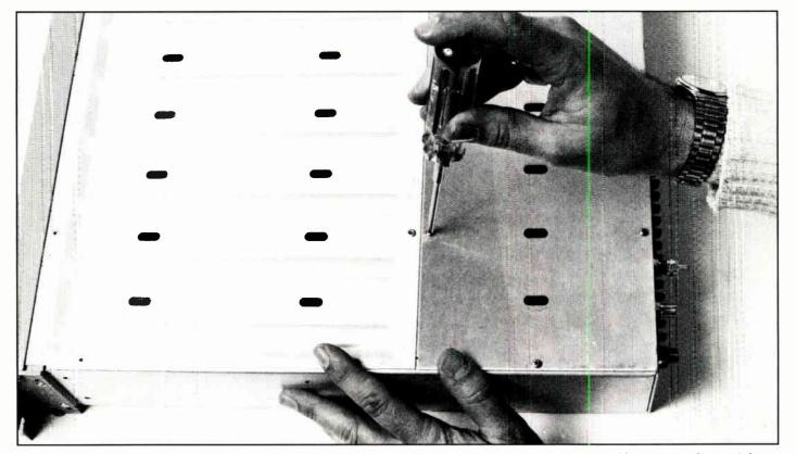
**Step 3:** To replace chassis connectors, begin by removing the lid that covers the rear compartment. Also remove the modules from the front of the chassis.
