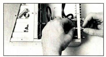
**Step 13:** Reconnect the RG-59 jumper to the connector making sure the center conductor goes in straight.
