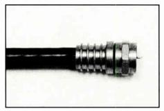
Step 6: Install the connector on the cable, leaving the braid folded back under the connector's crimp ring. When the connector bottoms out, the dielectric should be flush with the inside bottom of the connector.
