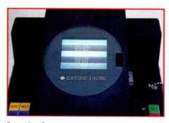
**Step 8:** Once the automatic process has been initiated, using a built-in camera and image processor, the machine positions the fibers, inspects the prepared ends, cleans them, and aligns the fiber cores in
