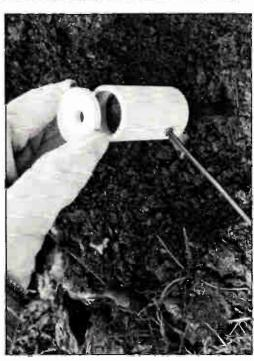
Photo 6: Place the cover on top of the mold.
