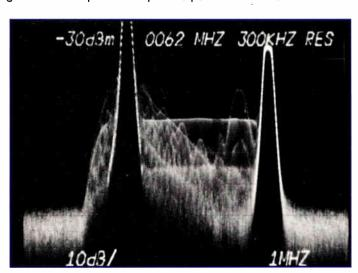
**Photo 3:** Modulator frequency response using the sin x/x video test signal.
