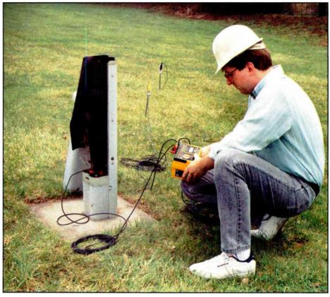
A technician checks grounds using a ground tester.
