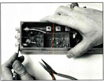
Step 3: Remove the module connector from the module.
