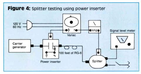
"Hum (modulation) on an addressable converter data carrier has been known to significantly reduce addressing reliability."
