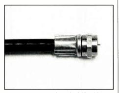
If your connector crimps look like this, you have either installed the wrong connector on the cable or used the wrong hex size on the crimping tool.
