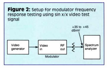
depth of modulation and output RF levels are correct. Photo 3 shows the in-channel response of the modulator using the sin x/x signal. Note that an analog display is necessary to resolve the  $\sin x/x$  response; RF input to the spectrum analyzer should be in the +35 to +40 dBmV range for a noise-free response display. Photo 4 is the same measurement made with the analyzer set to 2 dB per division.
