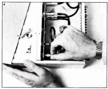
Step 8: Reconnect the RG-59 jumper to the connector making sure the center conductor goes in the connector straight.
