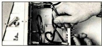
**Step 11:** Remove the nut that holds the barrel connector in the chassis and pull the connector out the back. Note that the barrel has flats on the threaded surface to prevent the connector from spinning in the chassis.
