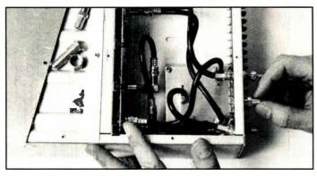
**Step 12:** Install the new connector from the outside; the retaining nut should be installed from inside the chassis rear compartment and wrench tightened.
