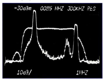
**Photo 2:** Processor frequency response on a digital storage display spectrum analyzer. A similar display can be obtained on analog storage analyzers.
