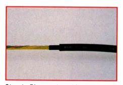
Step 1: Ring cut the cable sheath 10-12 feet from the end. Separate and remove the sheath from the cable. Fiber-optic splicing requires this extra length to accommodate splicing equipment and to allow for unanticipated remakes of cleaves or broken fibers.
