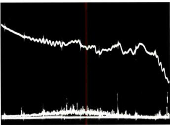
Structural return loss of reel of .750 1 GHz cable.
