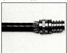
**Step 4:** Using the connector you will be installing, shape the dielectric as shown. Push the connector on "backwards" until it bottoms out at the braid.
