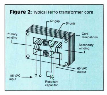
Efficiency will be the best at close to full load and low input line because most of the circulating VA is being delivered to the output load. Efficiency will be worse at nominal or high input line with less than full output load. Again, this is because of the large amount of circulating VA in the tank circuit that is not being used by the load and is subject to core loss and winding resistance losses.
