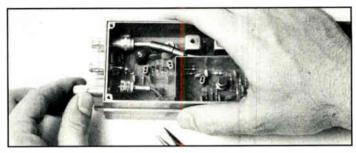
Step 4: Install the new connector and wrench tighten it.
