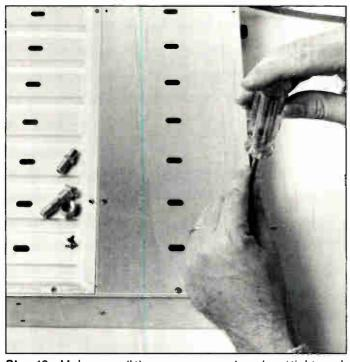
Step 16: Make sure all the screws are replaced and tightened.
