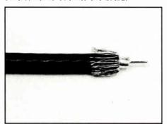
Step 5: Remove 1/4 inch of dielectric; be sure you don't nick the center conductor. This procedure will leave 1/8 inch of exposed dielectric and 1/4 inch of center conductor.
