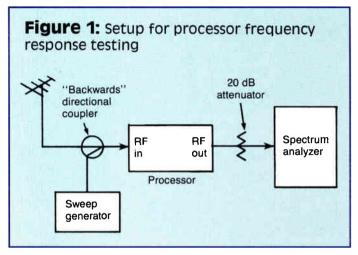
the off-air channel's carriers as markers while sweeping the processor. Furthermore, you can leave the processor's AGC turned on, providing you with an accurate sweep response in that mode. This also avoids interfering with adjacent channels while sweeping the processor.
