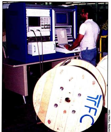
Production testing of 1 GHz cable requires upgraded test equipment and measurement techniques.
