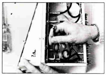
Step 4: Disconnect the RG-59 jumper from the back of the chassis connector. At this time check that the cable's center conductor diameter and length are correct.
