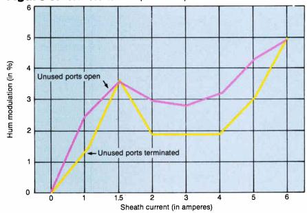
When circuit breakers trip or fuses open on individual phases of the utility distribution, increased neutral current results even if only momentarily. This condition can cause significant currents to flow in nearby CATV drops. Destructive tests indicate that the 28 gallium windings of these ferrite transformers will open at about 6 A. This translates to a total current of about 36 A impressed on a 100-foot RG-6 trishield drop by a potential difference of only 20 V-even less on shorter drops.
