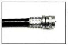
Step 7: Finish the installation with a hex crimp tool. Make sure the tool's hex dimension is the right one for the connector you are using, and don't use a worn-out pair of crimpers.
