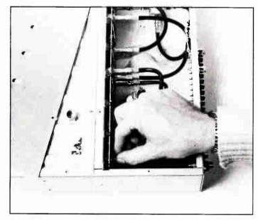
Step 6: Push the chassis connector through the front of the chassis.
