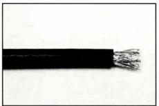
**Step 2:** Remove 3/8 inch of jacket, being careful not to cut into the braid.
