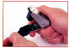
Step 6: Place the stripped fiber into a cleaving tool to cut the fiber end. Preparation of a perfect end face with a minimum of angularity is the most important step in the splicing process. End face quality directly affects the splice loss and mechanical strength of the joint.
