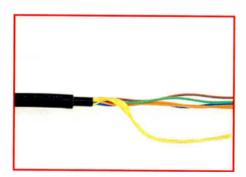
Step 2: Remove the wires, spacers, tapes and strength members from the cable, leaving the closure manufacturer's recommended length to secure the cable within the closure. Most fiber-optic cables are filled with a water blocking compound and
