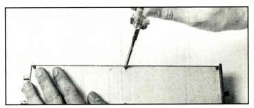
Step 1: Remove the six screws that hold each module cover in place.
