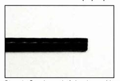
**Step 1:** Cut the end of the drop cable square with a sharp pair of cutters.
