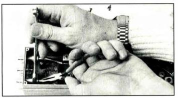
**Step 2:** To prevent twisting off the center pin of the RG-179 cable inside the module, grip the flat surfaces of the crimped retainer sleeve on the cable's F connector with needle nose pliers when disconnecting the cable from the module connector.
