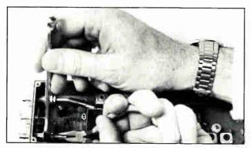
**Step 6:** Carefully reconnect the RG-179 cable to the module connector, holding the retainer sleeve with needle nose pliers while tightening the F connector.
