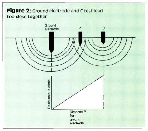
are placed too close to the ground electrode to be tested gross errors will result (see Figure 2). If the probes are placed far enough away from the ground system to be tested (this is said to be out of the sphere of influence of the rod to be tested) an accurate test can be made (see Figure 3).
