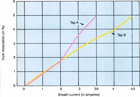
Figure 6: Test results of Splitter A
