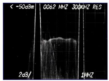
**Photo 4:** The same measurement from Photo 3 with the analyzer's vertical scale set to 2 dB per division.
