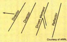
Figure 4: Basic log periodic dipole array maximum signal strength is off of the feed point end A yagi is a directive gain antenna that has a dipole as its driven or active element and parasitic elements that may include a reflector and one or more director elements (see Figure 3). Parasitic elements are not directly connected to the driven element or the transmission line, but instead are powered by close-proximity coupling to the driven element.
