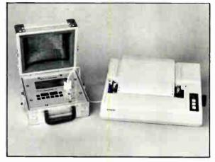
Designed for CATV and LAN. The CCR-4 cable radar gives a high resolution computer and graphic display, locates opens, shorts and impedance changes. Uses high resolution LCD with backlighting. Full memory that **c**an be stored by time and date. For a hard copy of the graphic display screen or the printed coordinate screen, the CCR-4 has an RS-232 port which enables a down load to various portable printers or directly to your PC. It is based on Time Domain reflectometry.
