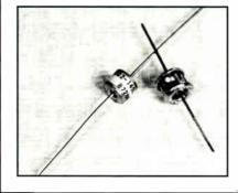
is the AC de-coupling chokes that are located in the input/output trunk ports and the feeder legs from the bridger output. Careful selection and use of these AC chokes that have a self resonance outside of the desired bandwidth will create the recovery of the needed return loss at the upper frequencies. The 300 MHz trunk station assemblies of yesterday can now be the 550 MHz fiber interface of tomorrow.
