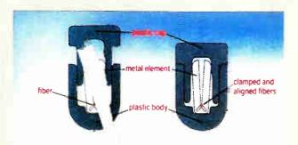
A simple, virtually flawless method for aligning the centers of two fibers. A splice that ensures transmission with a quick snap of the cap.
