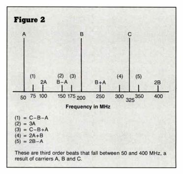
to produce sufficient distortion to be measurable. Check that you haven't driven the amplifier into compression by raising (or lowering) the carrier levels by 2 dB and ascertaining that the CTB product changes no more than 6 dB. From these results calculate what the three tone triple beat distortion will be at the levels you will be operating the system.
