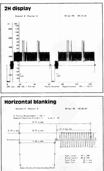
while not broadcast quality, a Commodore's output video is useable on a cable system. The accompanying table summarizes what was measured; unfortunately, the computer has no internal adjustments to vary any of these parameters.
