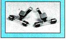
to a standard fuse body) was designed to replace the standard fuse links in areas of random fuse blowing. These Amazon breakers have been extremely useful in high lightning strike areas. Another useful fix for surge problems is the AmpClamp, a small circuit that is installed in line power inserters (see "In the good ol' summertime" by Roy Ehman, May 1989 *CT*.)
