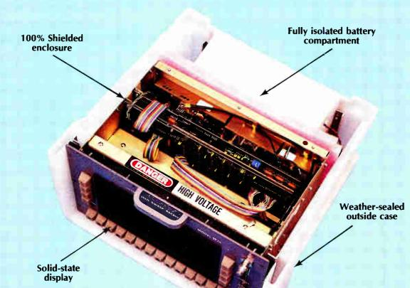
Reliability built into a CALAN, Inc. Model 1776 Sweep Receiver is very apparent from the outside: the totally weather-sealed case; the ruggedized overall construction; the moisture-sealed key covers on the front panel.
