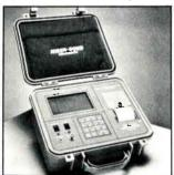
Model 1210 Universal TDR, Cable Fault Locator
